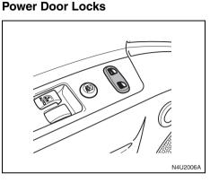
If your vehicle has this feature you can unlock or lock the doors on your vehicle using the driver's door lock switch. Push down the front part of the switch to unlock the doors. Push down the back part of the switch to lock the doors.
